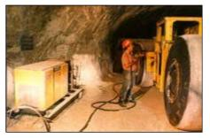
All equipment used in the mine, such as this transport vehicle, must be cleaned of potassium salt dust regularly. This is accomplished by intensive blowing. The air needed for this work is supplied by an AS 35 oil-cooled screw compressor from KAESER.
